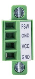
☑ Please ensure no external voltage is applied to PSW! This could cause damage.Use the terminal block to connect the Edge Gateway to a 12-24V DC power source.
